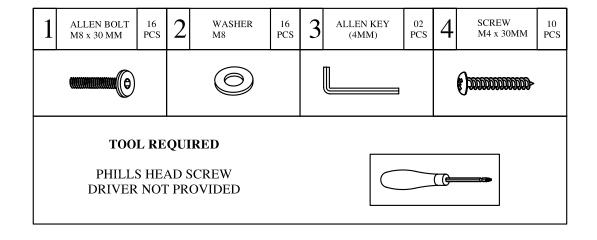
FIX ONE OF THE SIDERAILS (C) TO THE HEADBOARD (A) USING ALLEN KEY (3) AND ALLEN BOLT (1) AND WASHERS (2). DO NOT TIGHTEN BOLTS COMPLETELY UNTIL ASSEMBLY IS COMPLETED
