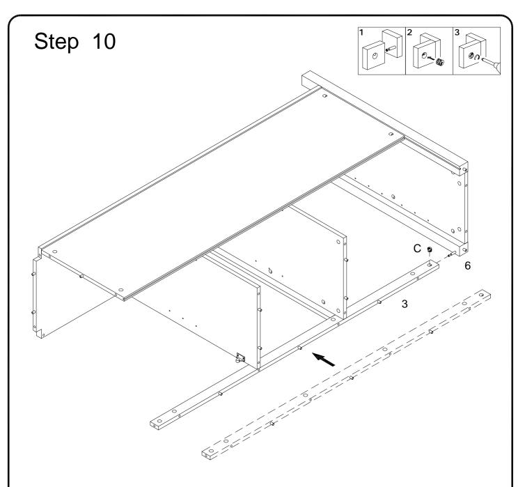
Using cam lock (C) secure part (6) to part (3) with Philips head screwdriver as per diagram.
