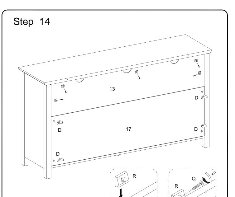
Using screw (Q) secure plastic wedge (R) with Philips head screwdriver ,then place stickers (D) cover the holes as per diagram.
