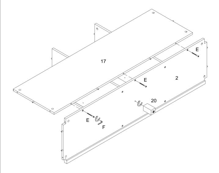
Using screw (E) attach part (2) to part (17) with hex key (F),and attached part (20) to part (2) as per diagram.
