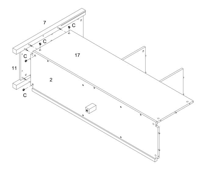
Using cam lock (C) secure parts (7,11) to parts (2,17) with Philips head screwdriver as per diagram.
