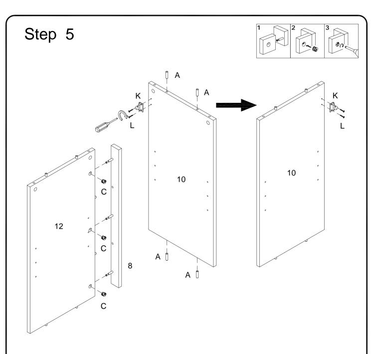
Insert wooden dowel (A) into part (10), using screw (L) attach magnetic touch (K) to part (10) and using cam lock (C) secure part (8) to part (12) with Philips head screwdriver as per diagram.
