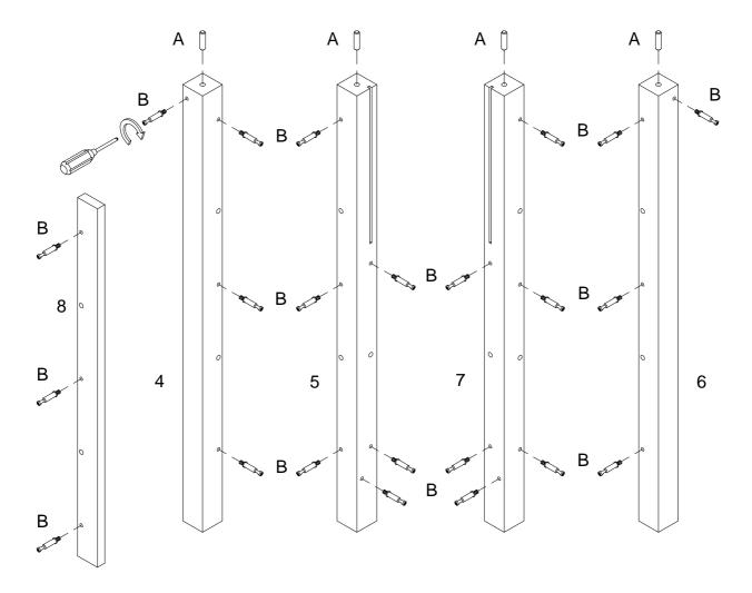
Insert wooden dowel (A) into parts (4,5,6,7), then secure cam bolt (B) into parts (4,5,6,7,8) with Philips head screwdriver as per diagram.
