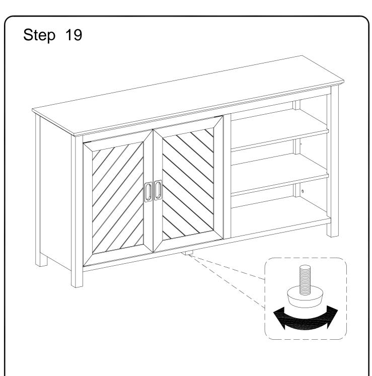
If necessary, adjust the pre-attached Floor Levelers at the bottom of legs to level the unit.
