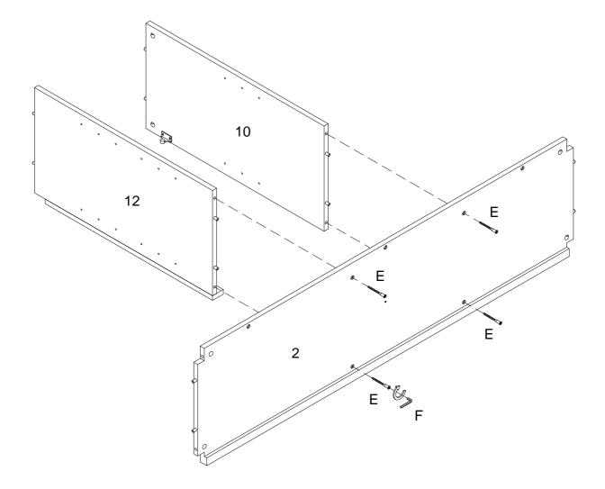
Using screw (E) attach part (2) to parts (10,12) with hex key (F) as per diagram.
