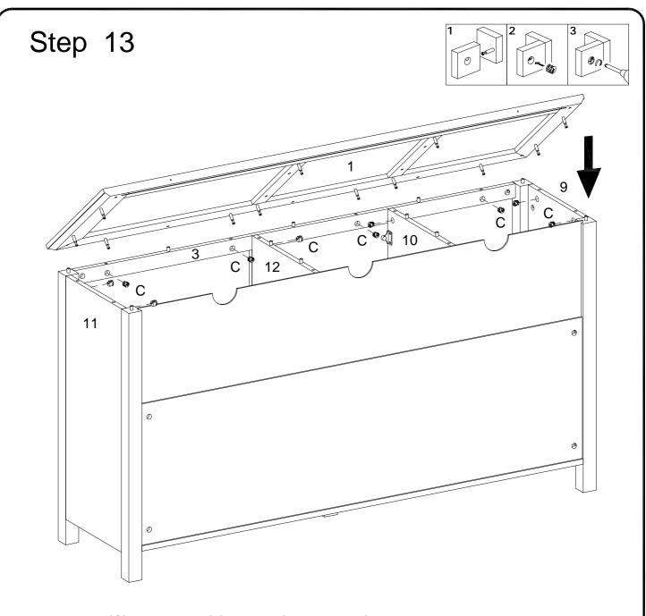
Using cam lock (C) secure part (1) to parts (3,9,10,11,12) with Philips head screwdriver as per diagram.
