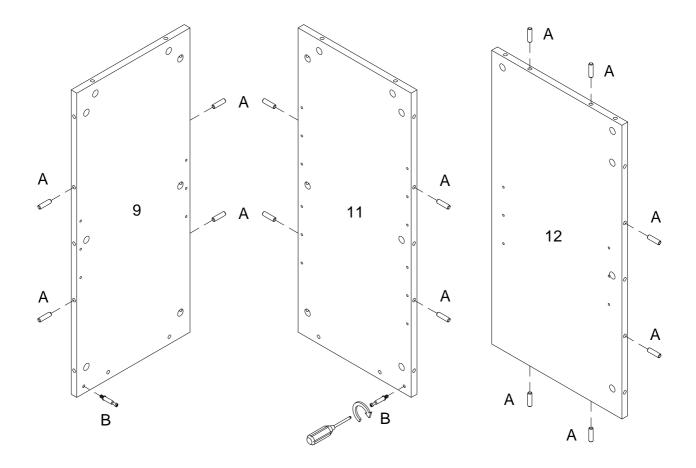
Insert wooden dowel (A) into parts (9,11,12) as per diagram.
