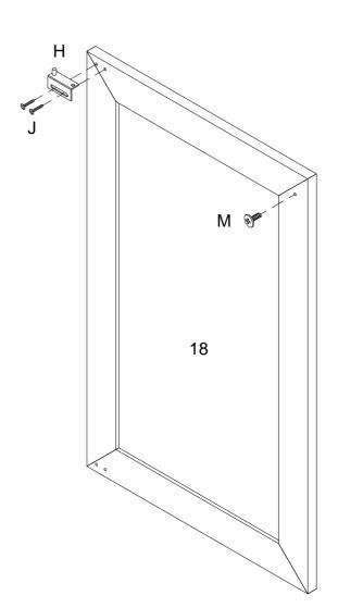
Using screw (J) attach door hinge (H) to parts (18),(G) to part (19), and secure bolt (M) into parts (18,19) with Philips head screwdriver as per diagram.
