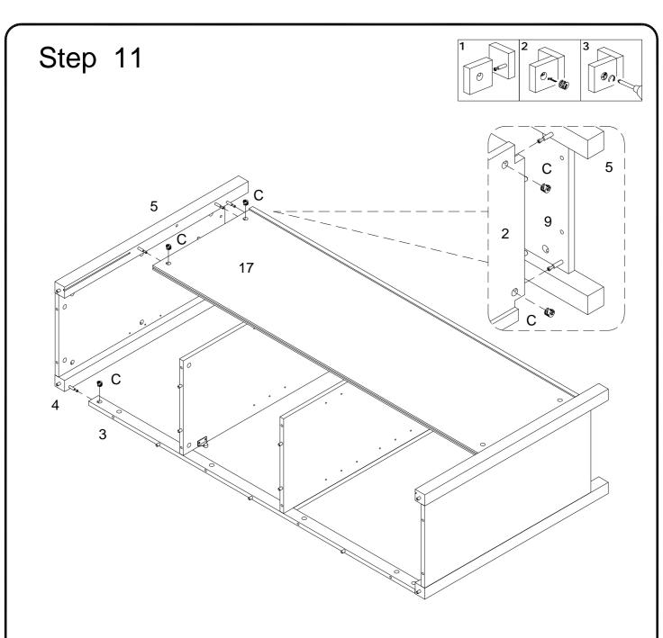
Using cam lock (C) secure part (4) to part (3) ,parts (5,9) to parts (2,17) with Philips head screwdriver as per diagram.
