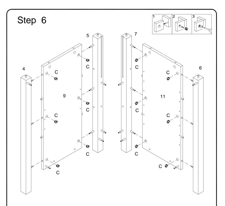
Using cam lock (C) secure parts (4,5) to part (9),parts (6,7) to part (11) with Philips head screwdriver as per diagram.
