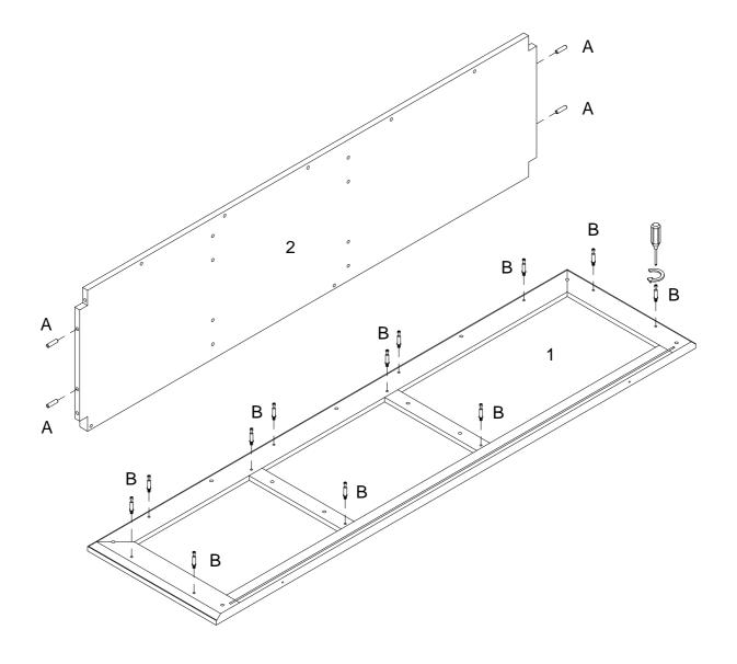
Insert wooden dowel (A) into part (2), then secure cam bolt (B) into part (1) with Philips head screwdriver as per diagram.
