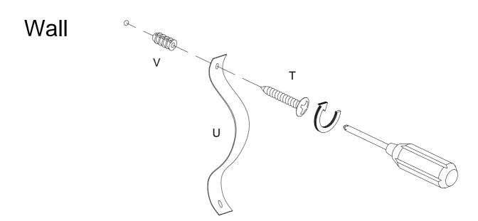
Using screw (T) attach Velcro strap (U) into Nut (V) to wall with Philips head screwdriver as per diagram.
