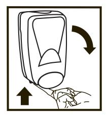
**1.** Press button on bottom of dispenser to open cover. Alternatively, use separate key tab to unlock cover.
