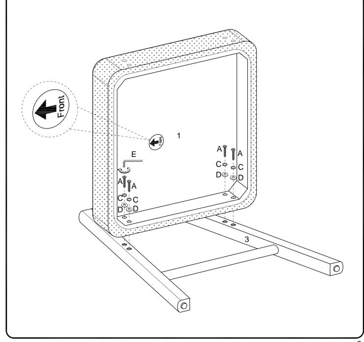
Now, repeat the process for the other side. Secure the Stool Seat (1) to the Right Leg Frame (4) using the Bolt (A), Lock washer (C), and Washer (D). Tighten with the Hex key (E).
