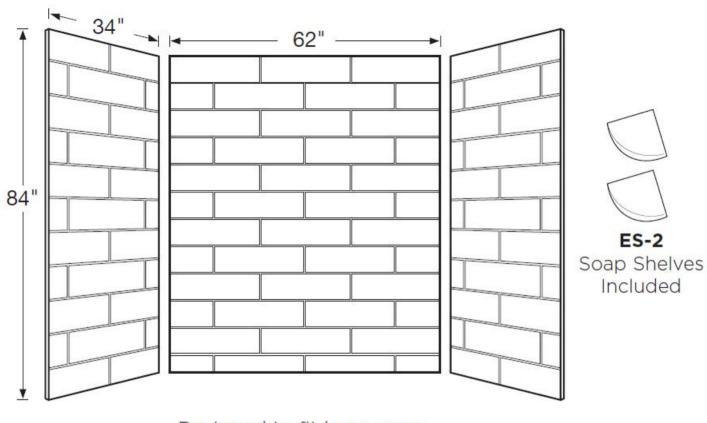
Designed to fit base areas 34" deep or smaller x 62" wide x 84" high or smaller (864 mm x 1575 mm x 2134 mm)
