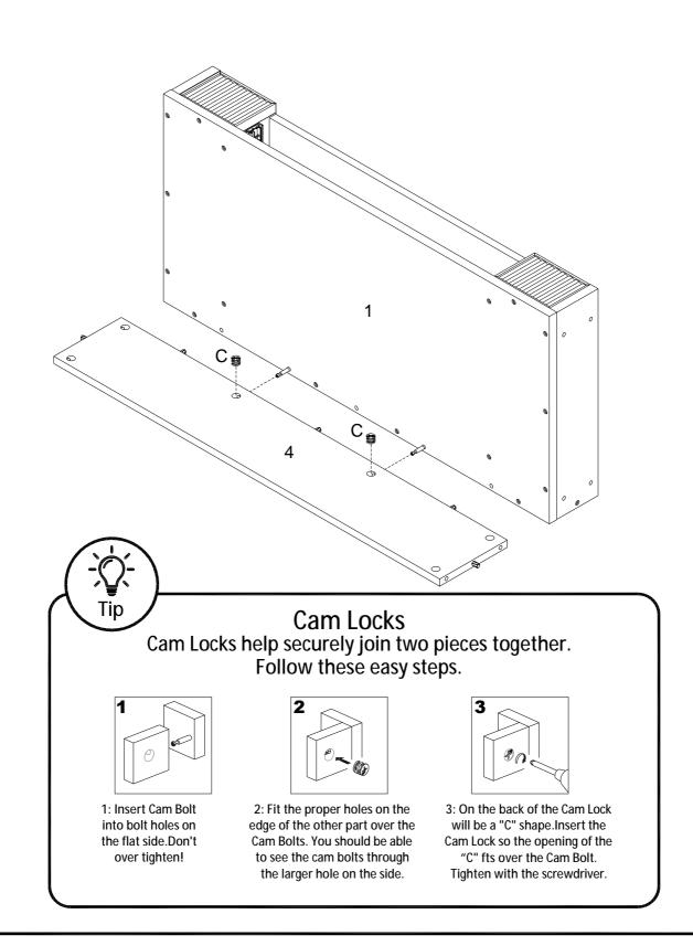
Attach the Left Panel (2) to the Desk Box (1) using 30mm Bolts (G). Bolts go through the inside of the Desk Box, into the Left Panel. Then, attach the Left Panel (2) to the Back Panel (4) and Support Panel (5) using Cam Locks (C). Secure with a screwdriver.
