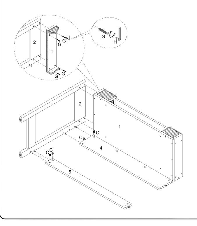
Repeat the same steps to attach the Right Panel (2) to the Desk Box (1) using 30mm Bolts (G). Bolts go through the inside of the Desk Box, into the Left Panel. Then attach the Right Panel (2) to the Back Panel (4) and Support Panel (5) using Cam Locks (C). Secure with a screwdriver.
