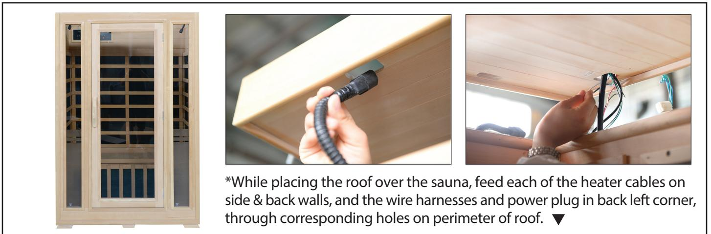
\*While placing the roof over the sauna, feed each of the heater cables on side & back walls, and the wire harnesses and power plug in back left corner, through corresponding holes on perimeter of roof. ▼
