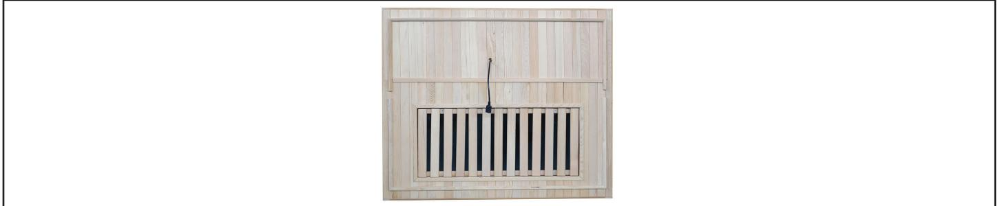
2. Place the BACK PANEL on the FLOOR PANEL, lining up the BACK PANEL against the floor trim piece on the backside of the FLOOR.
