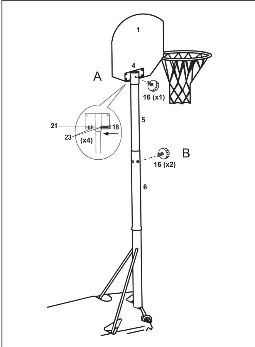
A. Place Connecting Plate (4) over top of Tube (5), and secure in place with one Knob Bolt (16) screwed into threaded hole on back of tube 5.
