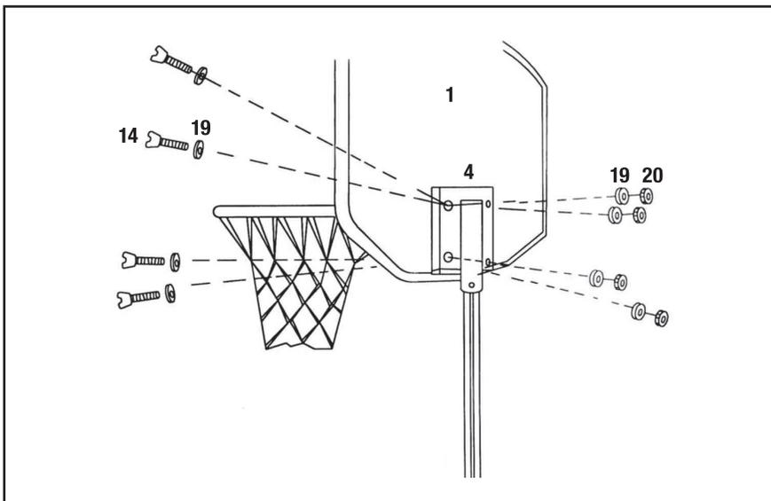
Use four Rim Bolts (14) to attach Basketball Rim (2), from front side, thru holes in Backboard (1) and to Connecting Plate (4), on back side. *Note: Use Washers (19) on both sides.* Tighten bolts (20)
