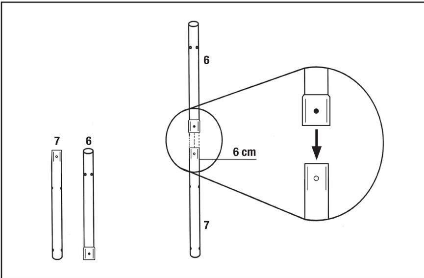
Snap Tube (6) and Tube (7) together using button lock into hole. Make sure you have a firm connection.
