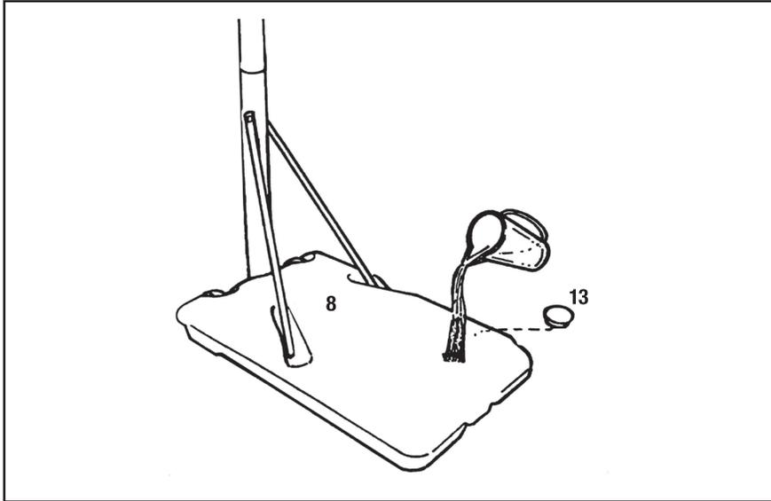
Remove Base Filler Cap (13) and fill Base with water. Replace cap
