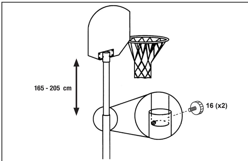
Knob Bolts (16) can be loosened and tightened to hold backboard at desired height by moving tube 5 up or down.
