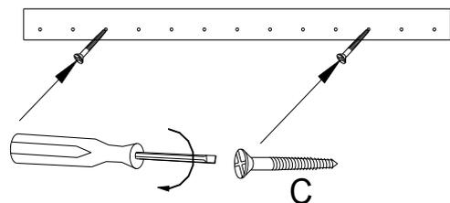
**It is recommended that the cleat (B) be securely screwed into the studs for stability.**
