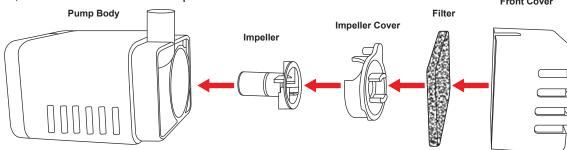
Press down on the top of the front cover and pulling it off by the sides.
