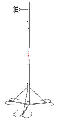
Place Top Pole (E) onto the bottom pole.
