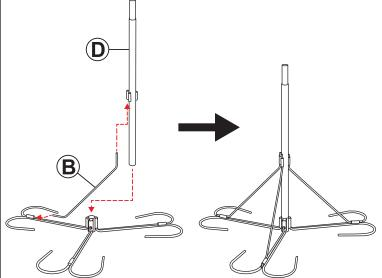
Install Legs (B) into the feet and Bottom Pole (D). Tighten the bolts on the base bracket.
