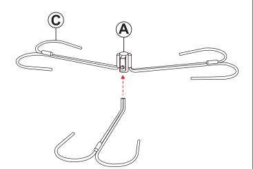
Loosen the bolts on Base Bracket (A). Install three Feet (C) into the base bracket.
