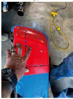
5. Place template on bag lid and drill a screw in either one of the two center holes. Before drilling in the second screw, double check that the template is still in position and has not shifted. After that has been confirmed, drill the second screw into position. Now your template should be in place and have no visible gaps between the template and the bag lid.
