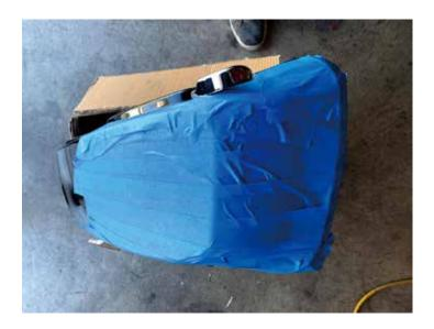
4. Test fit the template to make sure you have all painted surfaces covered with masking tape and that the template can be firmly mounted with no gaps.
