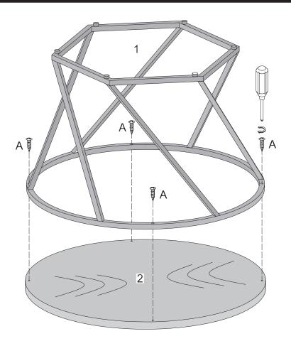
Secure the screw (A) to the metal base (1) to the table top (2).
