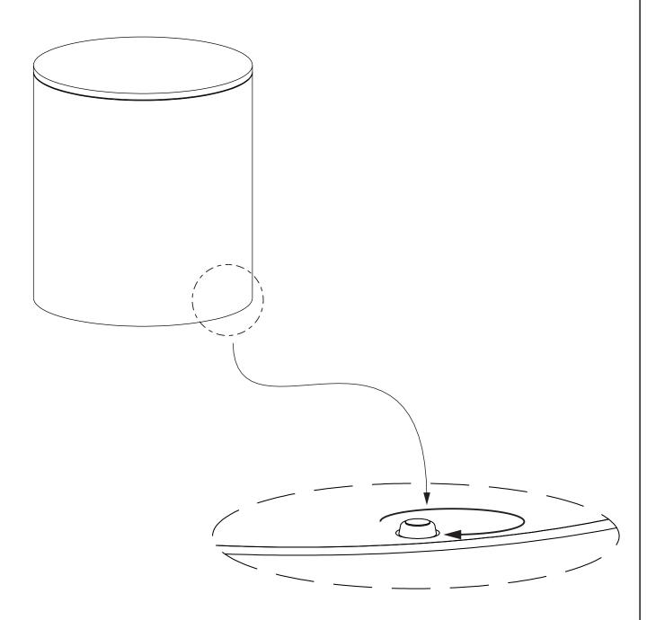
**NOTE:** Levelers on the bottom can be adjusted if floor is uneven.
