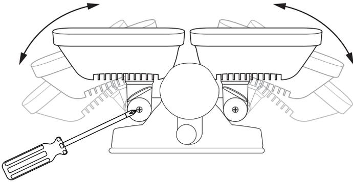
2 Adjust Flood Light Heads up and down.
