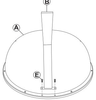
Loosely fasten four Legs (B) to Fire Bowl (A) by hand-tightening M6x15mm Bolts (E).
