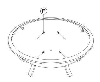
Align the holes inside the fire bowl with the middle of Leg (B) and secure using M6x12mm Bolts (F). Finish tightening bolts from Step 1.
