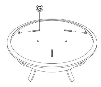
Install three Grub Screws (G) into the inside rim of the fire bowl.
