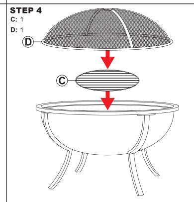
Place Log Grate (C) into the fire bowl. Rest Spark Screen (D) on the grub screws.
