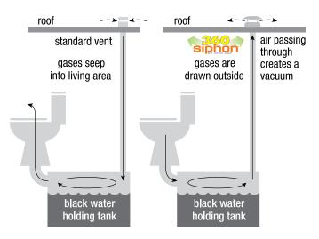
RV vent cap upgrade eliminates odors at the source by creating an updraft to exhaust odors through the roof vent
