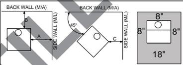
**IF THE STOVE IS TO BE INSTALLED ON A COMBUSTIBLE FLOOR, IT MUST BE PLACED ON AN APPROVED NON-COMBUSTIBLE HEARTH PAD THAT EXTENDS 8" (200MM) BEYOND THE STOVE SIDES AND BACK AND 18" (455MM) TO THE FRONT.**
