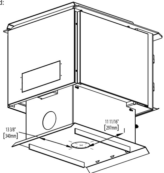
If possible connect the air intake at the pedestal's back or bottom to the outside with a 4" (102mm) diameter fresh air kit available at your local authorized dealer / distributor.
