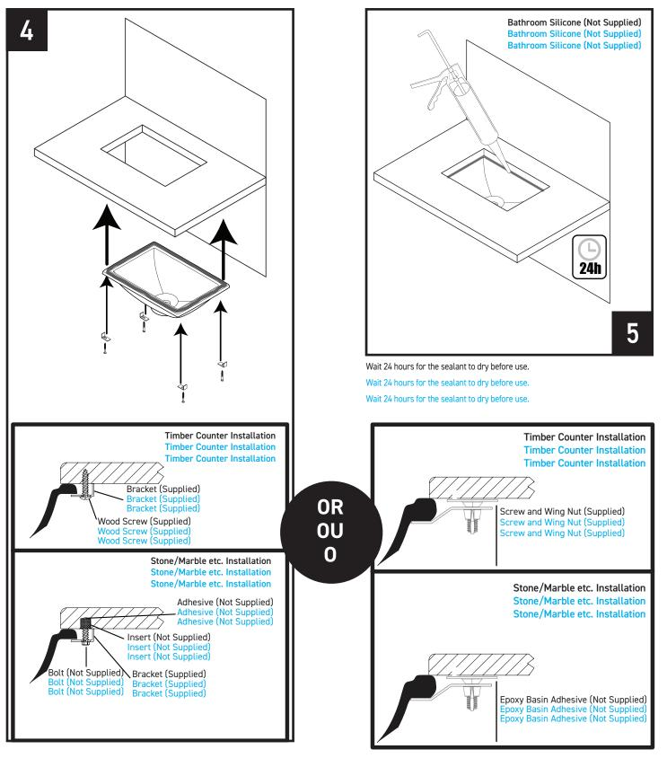
Once the sealant is applied, lift the sink up and press firmly on the underside to ensure there is a tight seal between the sink and counter. Based on the counter material, ensure you use the appropriate hardware as shown above to mount the sink in place.
