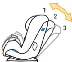
**Only** use semi-reclined **Position 2** if **necessary** to install the booster seat flush against the vehicle seat back.
