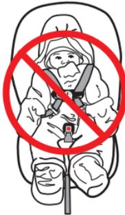
**DO NOT** mistake comfort for safety. The harness system **MUST** be snugly adjusted.
