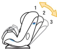
For children **who cannot sit up unassisted**, the **Rear-Facing Level Line** on the car seat **MUST** be parallel with the ground using either **Position 3 or 2**.
