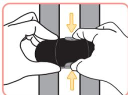
**For magnetic chest clip:** Hold the chest clip with both hands and press in on the top and bottom buttons with your index finger and thumb as shown.
