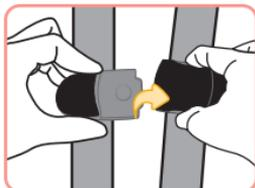
While holding the buttons in, pull the right (top) half of the clip apart from the left (bottom) half to release the magnet and separate the chest clip.
