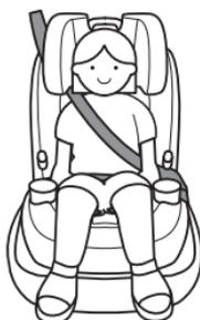
Check periodically to make sure your child has not moved out of position and loosened the shoulder belt.
