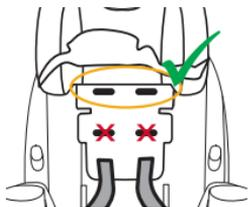
**If the harness straps have been removed from the splitter plate, chest clip & buckle, follow steps 9-11 in this section & the info box on page 52 to rethread them.**
