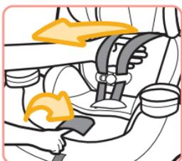
Push down on the harness release lever (through the opening in the pad) while pulling out on the harness straps as shown.
