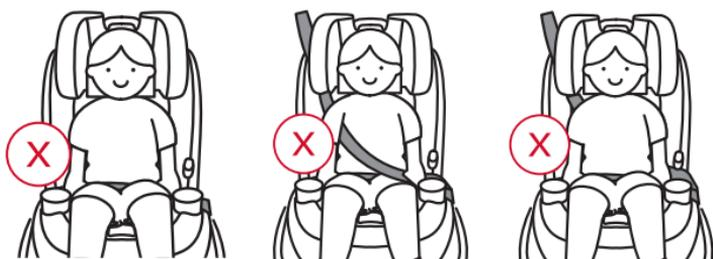
**DO NOT** use only the lap belt when using this seat as a booster seat. The shoulder belt **MUST** always be adjusted snugly across the child's chest.
