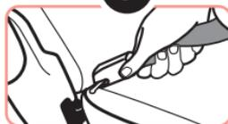
Fasten one lower anchor belt connector to the anchor located in the vehicle seat bight. Repeat for other side of car seat.
