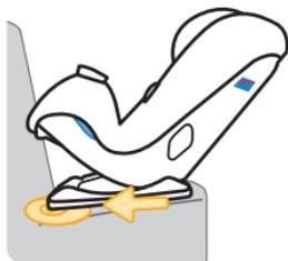
Only if necessary, you may place a tightly rolled towel(s) or foam pool noodle(s) under the front of the car seat base to help make the **Rear-Facing Level Line** parallel with the ground.
