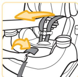
Push down on the harness release lever (through the opening in the pad) while pulling out on the harness straps as shown.
