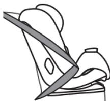
**Keep the booster seat securely belted even when unoccupied.**
