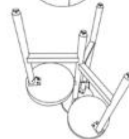
Fix Bottom Shelf with small Leg use small Allen screws in bottom side and large Allen screw in side leg
