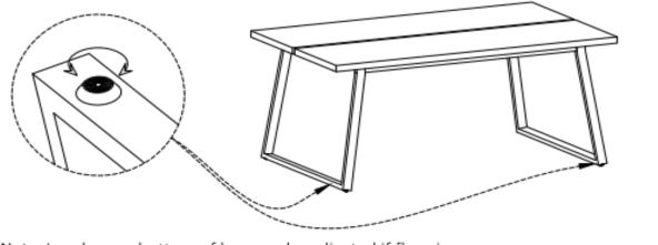
Note: Levelers on bottom of legs can be adjusted if floor is uneven.
