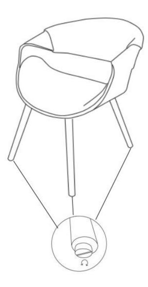
Place Chair on a flat level surface to ensure it is level. If it is uneven, adjust the leg levelers on the bottom of the legs.
