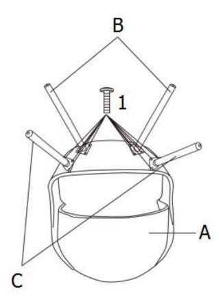
Attach the Front Legs (B) and Back Legs (C) to the Seat (A) with Allen Key Screws (1). Use Allen Key (2) to tighten.
