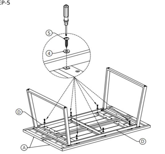
1. Use six Phillip Screws Round Head (5) and six Washers (4) to secure part (A) and (D).
