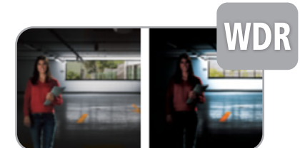
Wide Dynamic Range improves image quality by balancing dark and light areas in an image
