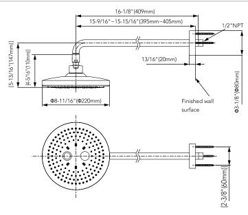
Note: The unit of above dimension is inch (mm); the dimension in [] is for reference only. Shower arm and mounting bracket are not included.
