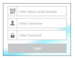
Input the serial number (click on the tool bar at the bottom of the live preview interface to see the serial number of the DVR), user name (the user name of the DVR, *admin* by default) and password (the password of the DVR, *123456* by default) of the DVR, select the display language on the top right corner of the interface and then click "Login" button to go to the web client interface.
