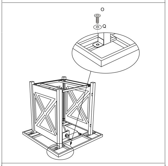
4.Attach the assembled base to the bottom of top using 4pcs of screws (O), and 4pcs M6 washers(Q), make sure the panel (L) faces the valve stem. Tighten all screws.
