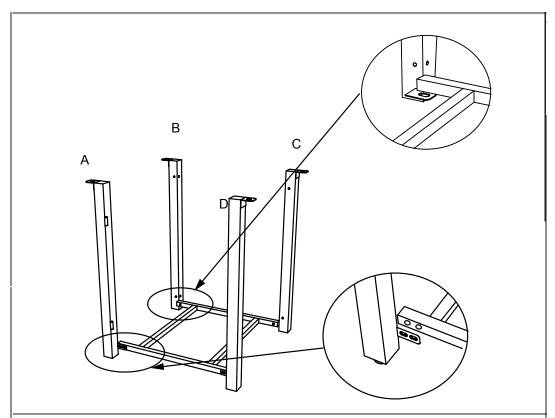
1.Connect the tank holder/base (I) With table Lets(A/B/C/D) by 6pcs screws (O) and 6pcs M6 washers(Q)
