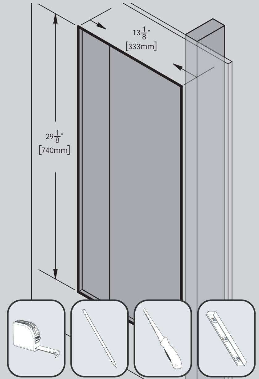
**2** Ensure unit is level, and use appropriate mounting hardware (4) to secure unit to support brackets (supplied by installer). Ensure alignment on plumbing connection is positioned into the 1/4" hole.
