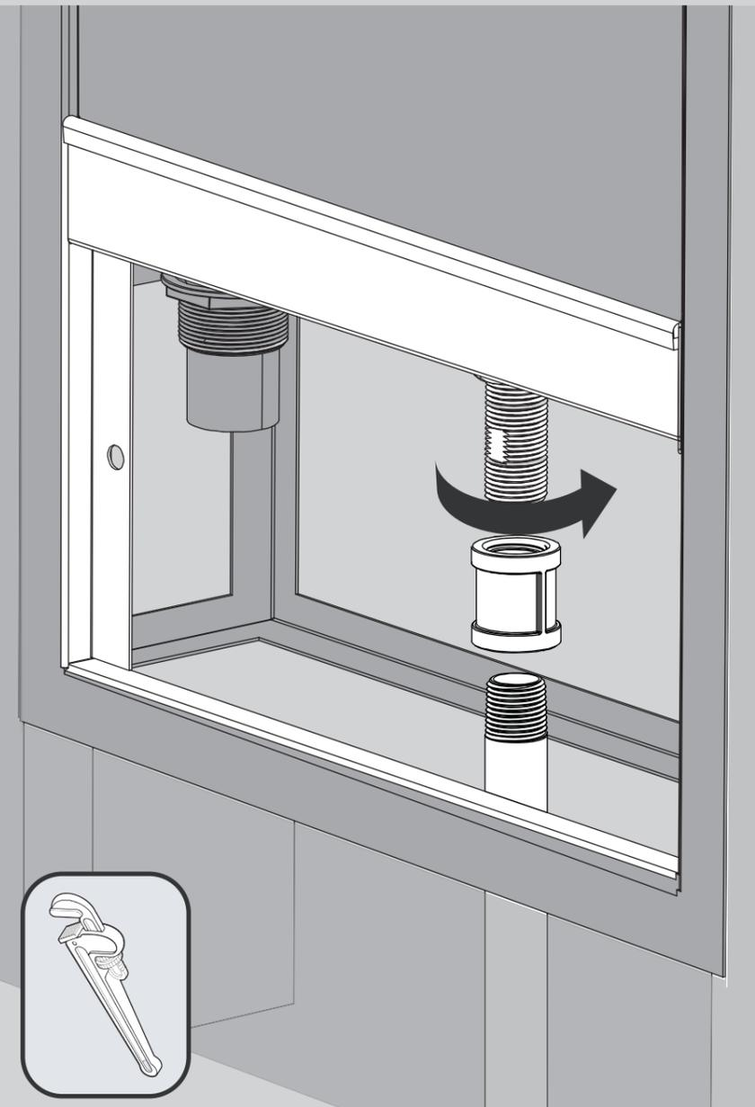
**4** Make appropriate drainage connections in compliance with local and/or national plumbing codes.
