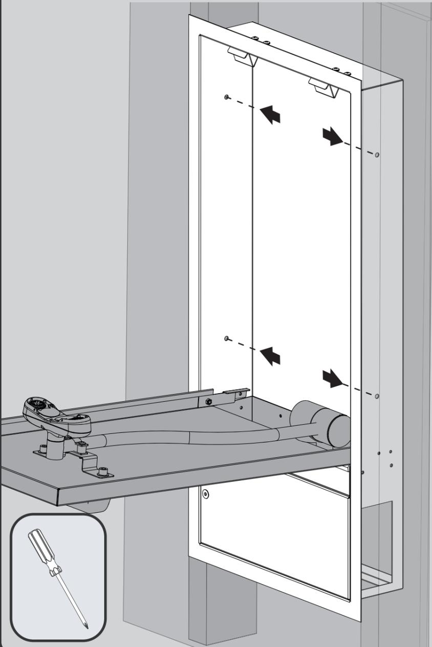
**3** Open lower access panel of cabinet. Install connection to inlet of Swing Activated Valve. Wrench tighten.
