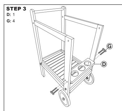
Align Bottle Holder (D) with the front of the side panels and loosely fasten using four M6x35mm Bolts (G).
