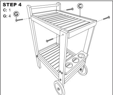
Align one Tray (C) with the top mounting holes on the side panels and firmly securing using four M6x35mm Bolts (G).
