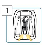
Remove Lower Anchor Belt from Storage Attachments
