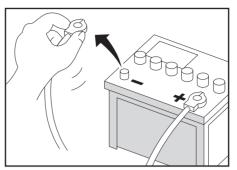
To avoid potential shorts in the electrical system, be sure to disconnect the (–) battery cable before installation. Use this unit with a 12-volt battery and negative grounding only. Failure to do so may result in a fire or malfunction.
