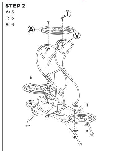
Loosely secure each Tier (A) to the side panels using two Bolts (T) and Nuts (V).
