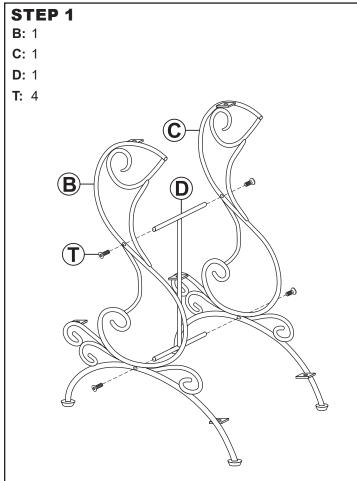
Loosely secure Center Bar (D) to Left Panel (B) using two Bolts (T). Then, loosely secure Right Panel (C) to the center bar.
