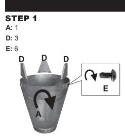
Place Main Body (A) upside down. Secure Leg (D) to the inside of the main body using two Bolts (E). Repeat to secure the remaining two legs.
