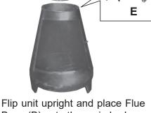
Base (B) onto the main body. Align the mounting holes and secure using three Bolts (E).
