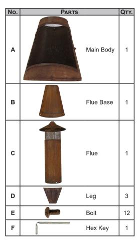
**NOTE:** The rust patina finish is a result of the alloy steel being exposed to water and oxygen. The color may continue to change over time. Help limit color change and further oxidization by covering or storing the fire pit when not in use.
