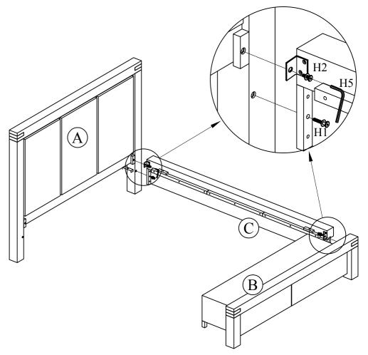
STEP 2: Repeat step 1 for the second side rail. Tighten all bolts completely with the provided Allen Key (H5)
