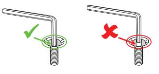
If the hex key is not fully inside the notch, the hex key could slip out, causing damage to the bolt head. Repeated hex key slipping will cause the notch to become rounded, making it difficult or impossible to tighten the bolt with the hex key.
