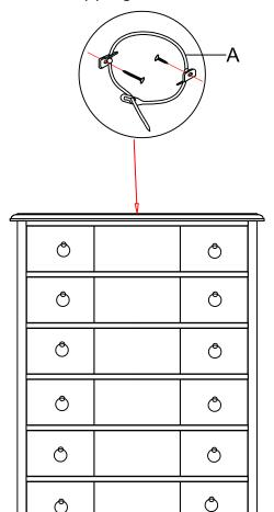
Anti-tip kit is included for use. We recommend installing for safety reason.
