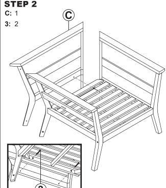
Loosely secure the underside of the seat to Backrest (C) by hand-tightening two M6x35mm Bolts (3).
