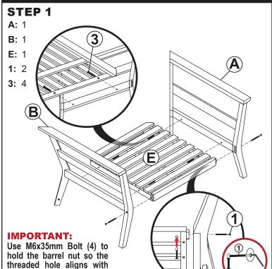
Loosely fasten Left Arm Panel (A) and Right Arm Panel (B) to the front of Seat (E) by hand-tightening M6x100mm Bolt + Barrel Nuts (1).
