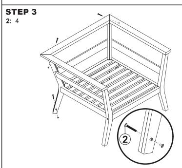
Secure the backrest to each arm panel using two M6x30mm Bolts + Caps (2) on each side.
