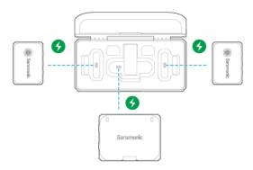
After recording, put the transmitter(s) and receiver back into the case for charging.
