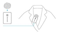
The transmitter comes with a windproof capsule. It can fit an extra fur windshield when you need to enhance wind protection outdoors or in a windy environment.
