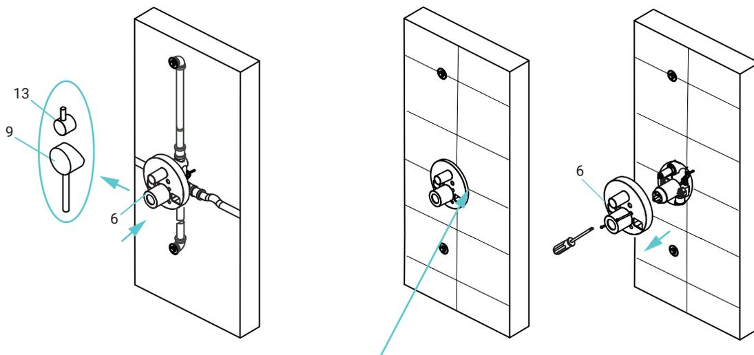
The tile surface should be 10cm lower than the black cover plate (6).
