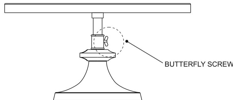
To adjust height of Cake Stand, loosen butterfly screw, position inner post to desired height and retighten butterfly screw.
