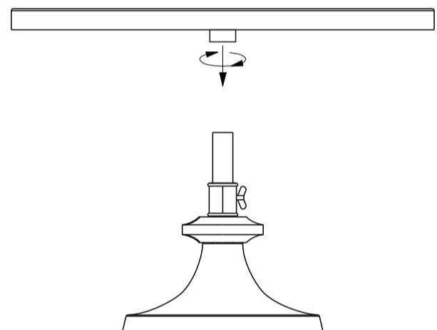
Fix Cake Stand Top to the Top of inserted pipe
