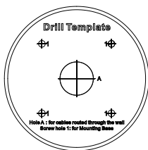
Figure 2-9 Drill Template of the Junction Box
