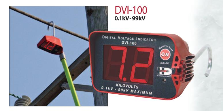
The DVI-100 is designed to be used on distribution systems in both overhead and underground applications and on transmission systems up to 161kV. The DVI-100 indicates voltage from 0.1kV - 99kV and is auto-ranging. Voltage is displayed on a large 2.25" LED display with a 2-digit readout. In addition, an audible alarm alerts the user to the presence of voltage above 100VAC. The DVI is auto shut-off and will turn off after 3-4 minutes of inactivity.
