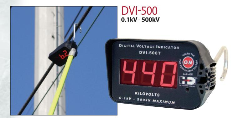
The DVI-500 is designed to be used on both transmission and distribution systems in overhead and underground applications. The DVI-500 indicates voltage from 0.1kV – 500kV and is auto-ranging with no range selector switch or settings required. Voltage is displayed on a large 1.45" LED display with a 3-digit readout. In addition, an audible alarm alerts the user to the presence of voltage above 100VAC. The DVI is auto shut-off and will turn off after 4 minutes of inactivity.
