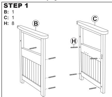
• Insert 4x JCBC M6x60 Grub Screw (H) into the inside of each Arm Panel (B, C).
