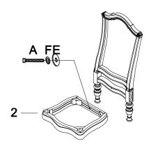
**STEP TWO:** Assemble the chair back(1) and the seat frame(2) securely using flat washers(E), lock washers(F) and bolts(B).
