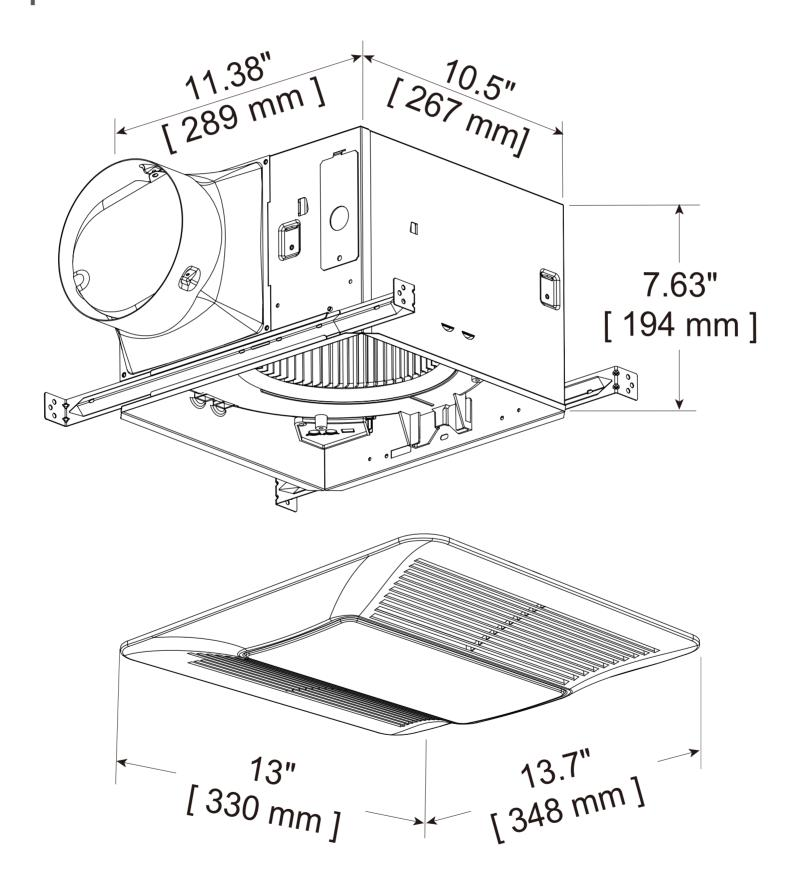
This fan can be installed to 13.8" - 24" between the joist or to I-joists, standard joists and truss construction.
