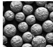
Conventional glass beads after sandblasting.
