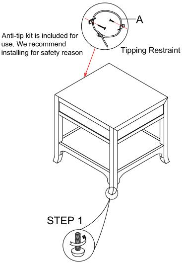
Adjust Leveler if needed to level table on uneven floor.
