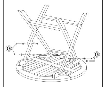
NOTE: Leg installation location may vary. For smaller size tables, install the inside legs on the outside of the of the blocks on the bottom of the tabletop.
