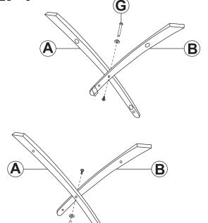
NOTE: Ensure the metal tab on Leg B faces inward, as shown in the top drawing.
