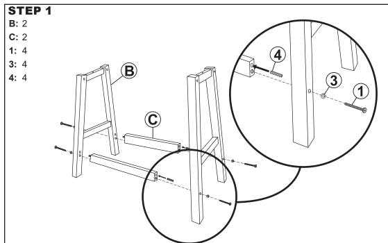
**IMPORTANT:** Do not install wood dowels into mounting holes with threaded inserts. Do not fully tighten hardware until after Step 2 is complete.
