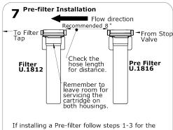
If installing a Pre-filter follow steps 1-3 for the second bracket taking into account the hose length supplied from the Pre-filter to the filter.
