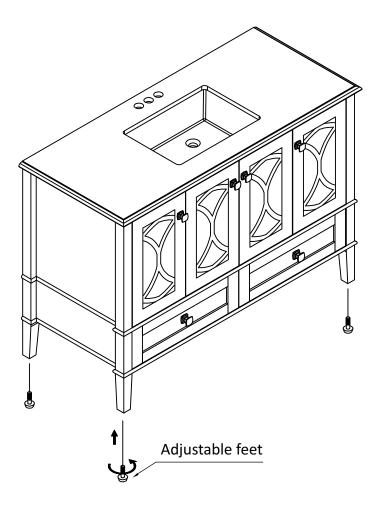
• If the floor is uneven, the adjustable feet levelers can be rotated to raise the vanity to the desired height.
